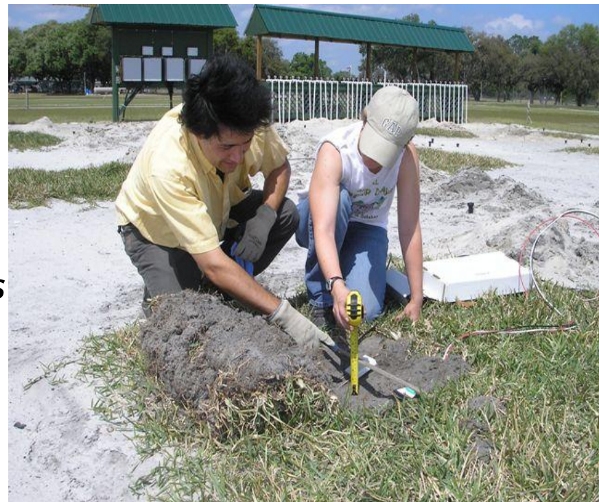
Soil moisture sensor (SMS) controllers
